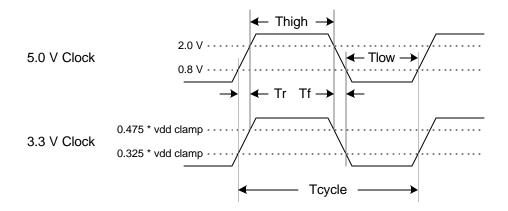
**PCI Clock Specification Timing Characteristics**
